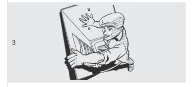
Trial fit the shower wall using masking tape to hold in position. Lightly mark the outside edge with pencil, this defines the required gluing area.
