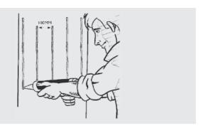
5. Apply adhesive beads in 4mm vertical lines spaced 110mm apart onto the wall lining over the shower wall area.
