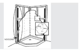
1. Fix Villaboard or WR plasterboard wall lining to framing
