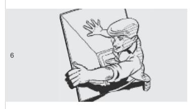
Place the shower wall onto the wall lining within10 minutes of applying the adhesive.
