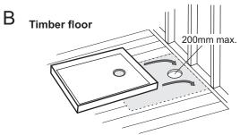
Install base on mortar bed or cement-based tile adhesive
