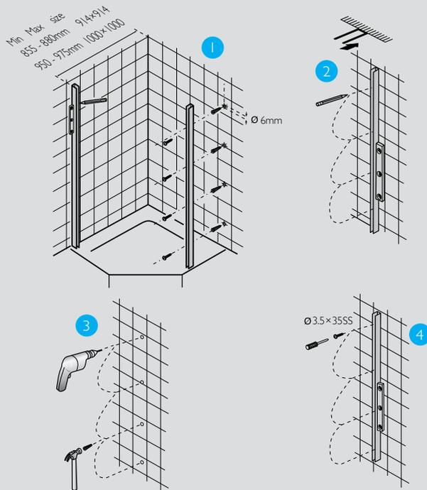
1 Measure your shower base/shower area. The measurement to the outside edge of the wall jambs(1) should be somewhere within the min and max size of the screen.
