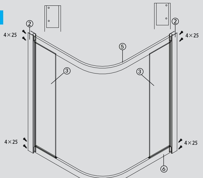
Screw the fixed panel extrusion(2) to the top and bottom rails. Please make sure that the location of the screw holes in the fixed panel extrusion line up with the holes in the top and bottom rails.
