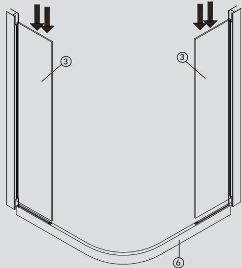
Push fixed panels(3) into seal that is located in the bottom rail(6). Make sure that the panel is firmly up against the fixed panel block(12) and fully inserted into the short seals(9). Hint-Wet the edge of glass & seal to make it easier to insert panel.
