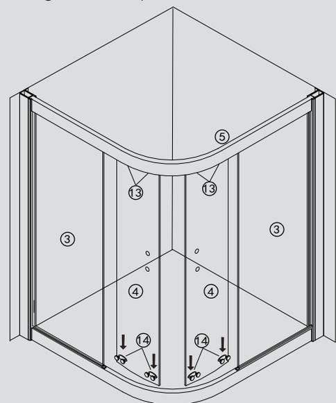
Adjust the sliding doors(4) using the screws located on the bottom of top roller assemblies(13). Adjust rollers so that the sliding doors (4) are parallel to the fixed panels(3) and parallel to each other. Note: Do not overtighten top rollers as this will cause the bottom rollers to jamb and or break.
