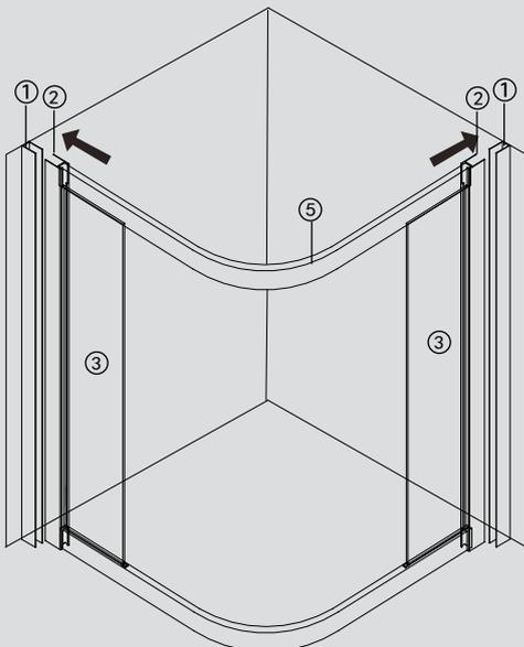
Adjust fixed panel extrusions(2) in or out on the wall jambs(1) so that the top rail(5) is horizontal and the whole screen sits square on the shower base/shower area.(B=C=D)
