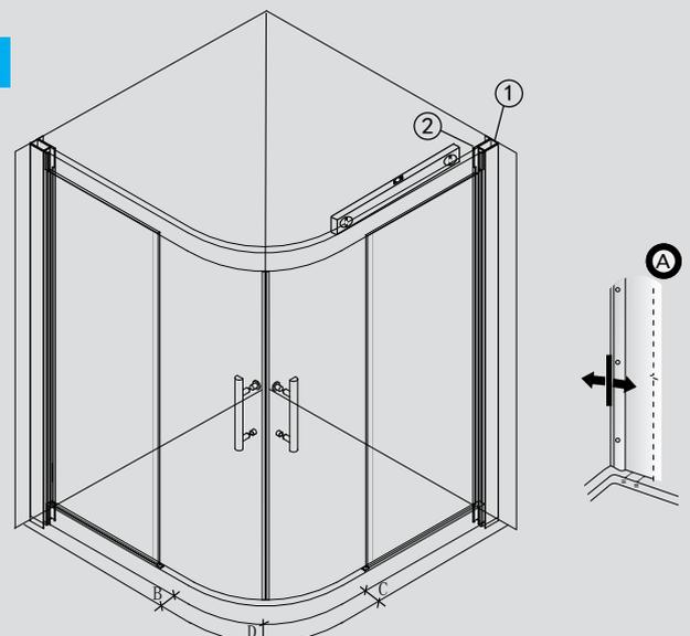
Adjust fixed panel extrusions(2) in or out on the wall jambs(1) so that the top rail(5) is horizontal and the whole screen sits square on the shower base/shower area. (B=C=D)
