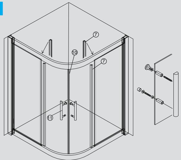
Gently knock the sealing strips(7) onto the fixed panels and doors. Attach the door handles(11) to the sliding doors making sure there is a washer between the glass and the handle. Gently knock the magnetic sealing strip(10) onto the sliding doors.
