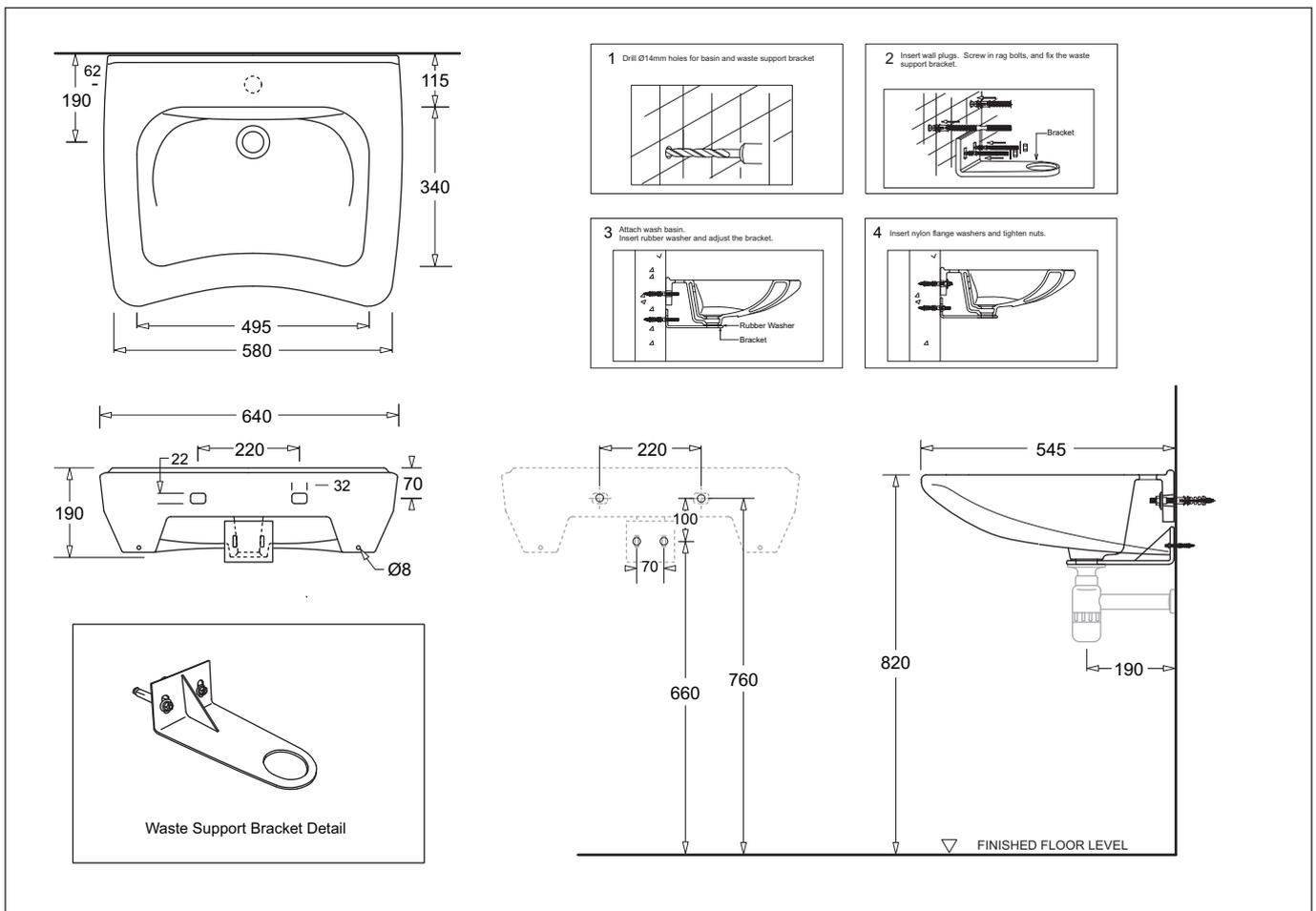
All dimensions are in millimetres and are subject to normal manufacturing variation of +/- 3mm on all surfaces.
